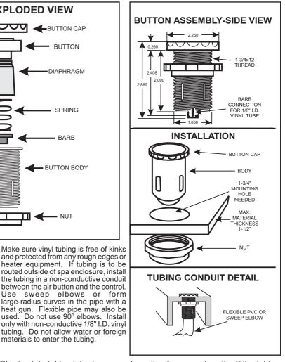
Blowing into tubing introduces condensation from your breath. If the tubing NOTE: must be blown out, use dry compressed air.
