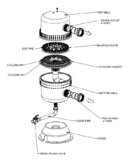
Incoming water is guided by a diverter plate so that it enters multiple hydro cyclones tangentially generating a strong centrifugal effect. This spins the sediment out to the hydro cyclone's wall and then spirals it down to the sediment chamber, while the cleansed water spirals upwards.
