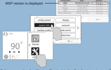
Before connecting the Wireless Terminal to the OmniLogic system, verify that you have the latest OmniLogic MSP firmware version. The firmware version displayed in "System Info" should be the same as the latest version available for download on the web. Follow the screens above to locate your MSP firmware version and go to Step 3 to find the latest firmware version
