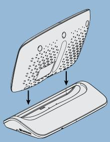
The following steps should be performed ONLY with the Wireless Terminal placed in the charging cradle, or after charging for at least 8 hours. If a firmware upgrade is needed, it must be completed while in the charging cradle.
